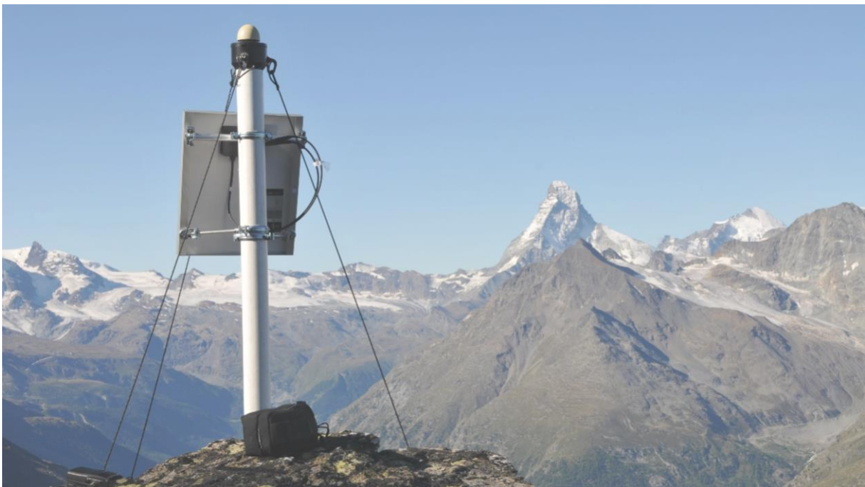
Figure 53: At the Matterhorn and further sites, Rock Glacier Velocity (RGV) ECVs are measured using permanently installed GNSS stations with daily resolution.
