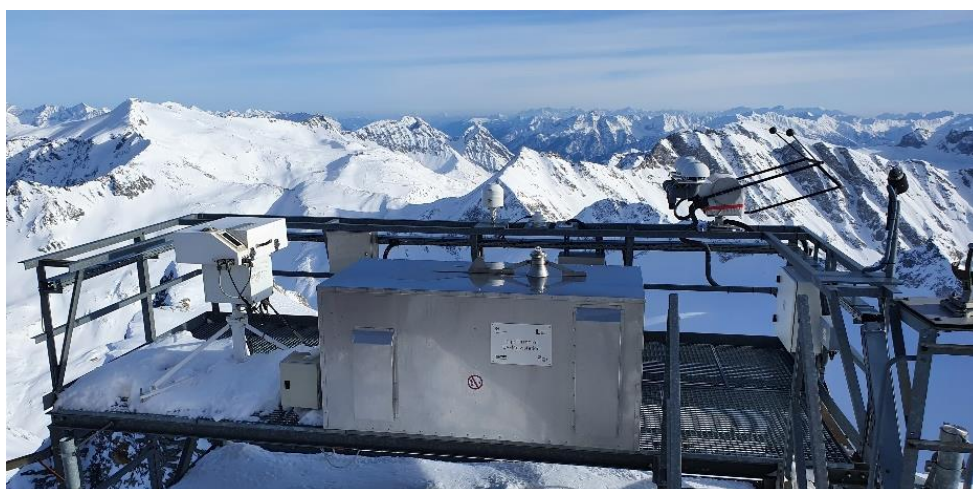
Figure 10: The Inge Dirmhirn UV Measuring Station at Sonnblick Observatory with Bentham spectral radiometer in foreground and the Brewer spectrophotometer in background.
