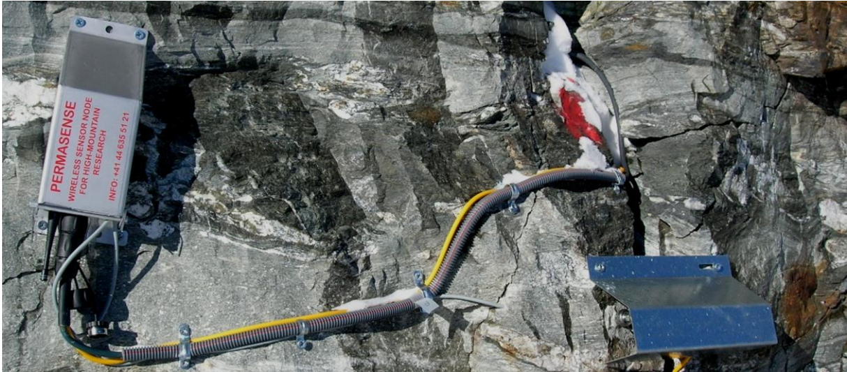
Figure 52: The main instrument used are small, battery powered wireless sensors.
